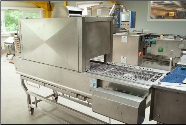
Clockwise from top left: Small Test Grill, Heater Cassette, Wire Belt, Insulated Undertrays, Hinged Insulated Access doors, Large Test grill
